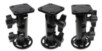
**215837 Pedestal Mount with wingnut** Pedestal mount 4", small teeth. Total length: 114 mm. Round base, square mounting plate 50x50 mm. Black.
