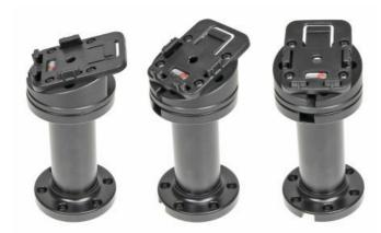
**215611 Pedestal Mount for cable entry** Pedestal mount 4", for cable entry. With angled top part 15° and MultiMoveClip. Height including top part: 135 mm. Black.
